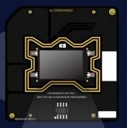
**OptoSelect**® chips use light to automatically move individual cells.
