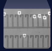
Cells are cloned and assayed in individual 500 pL or 1 nL NanoPen® chambers. Each pen is ~100,000 times smaller than a microwell.
