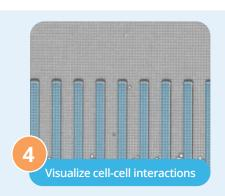
Precisely create individual cell-cell interactions by moving single cells with light.
